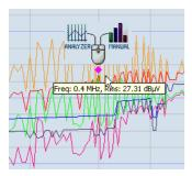
The Multi Marker function visible in fig. 2-3 can be used to highlight **Highest Peaks** detected in the graph window, in terms of a definable number of points for a specific Detector.
