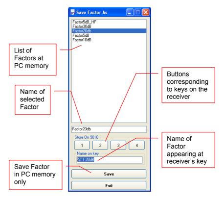
Select one between the four buttons in the field "Store On 9010" to automatically store the Factor at corresponding button on 9010. A progress bar will show status during storing and a pop-up window will confirm success of operation, resuming Name and Button assigned.
