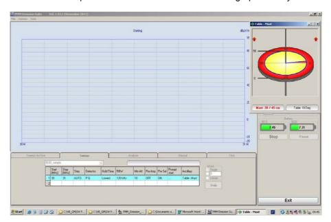
In the example above the red arrows indicate that the mast heigh is being augmented. The elevation range is between 0 and 55 cm.
