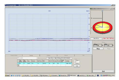
Above is another example in which the table is rotating counterclockwise. The bold blue radius indicates the actual angle of 149 degrees while the thin one shows the 190° end target.
