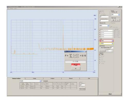
Example of failed IEC 62493 standard test.
