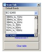
When a IEC 62493 test is to be run, the software must be operated in Sweep Mode.
