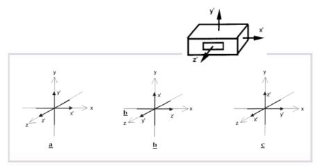
Fig. 3-4 EUT Orientations during Radiated Emission Test
