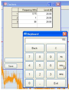
Up to 4 Factors can be added in Sweep, Analyzer and Manual Modes (see later description about Global Test Settings panel), where each one of them must be created through Factors function at first.
