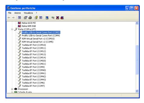
Check the value "COMx" mentioned between brackets at "USB-to-Serial Comm Port" items in the Communication Port tree and select corresponding "x" number in the Remote Link drop-down menu of PMM ES (Fig. 1-2).
