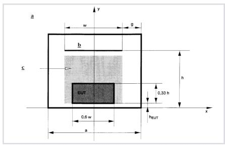
Fig. 3-6 GTEM Vertical section at EUT Position
