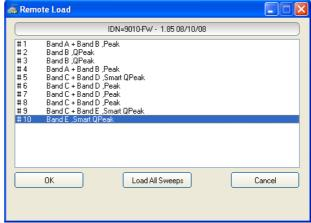
A label at the top shows the FW Release actually installed in the receiver. After selecting the sweep and confirming with "OK", a new window is opened, showing the sweeps already stored in the PC and proposing a default File Name "Auto\_01" for the sweep to be downloaded, which could be changed with a custom name:
