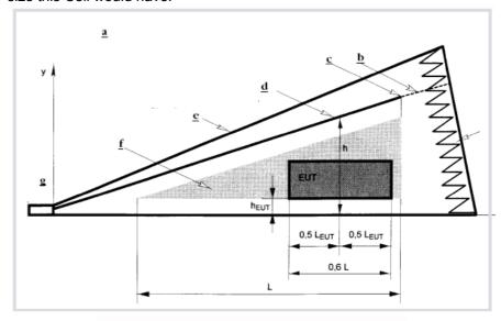
Fig. A.7a Side view CAPTION  $\mathbf{a}$ Side view b Load End of septum Septum (inner conductor) Chassis (outer conductor) Usable test volume Input port
